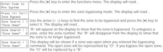
To exit the bypassing mode and return to the Ready state, press the [#] key.
